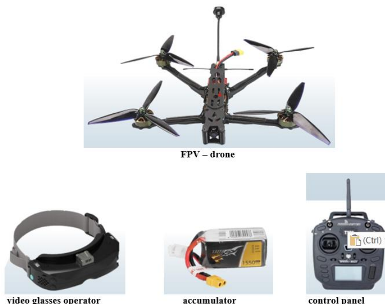
Figure 1. General layout of the FPV drone.
