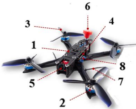
Figure 2 - general structure of an FPV drone.
